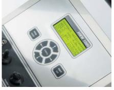
The temperature of the heating wedge is kept at up to 500°C with maximum precision, based on the specs of the used material, after the nominal temperature and the material characteristics for the imminent welding job were entered. The newly developed monitor for current flux to the heater cartridge ensures continuous temperature control. A possible current failure gets detected immediately and a plain-text alert shows on the high-res temperature range-extended character display.
