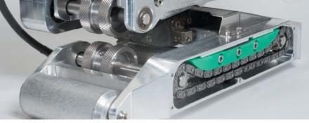
The welder is equipped with a drive system that does not require any maintenance and ensures fast and reliable "weld-wise" movement throughout the process, including for foils up to 3.5 mm (4 mm) thick, at a maximum speed of 6.00 m/min. Of course, the overlap of the two-piece joint reaching 15 mm and the in-overlap channel comply with the applicable DVS standard.
